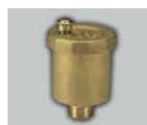
Automatic Air-Vent Valve Solid forged brass body Max temperature: 200°C Max working pressure: 10 bar
