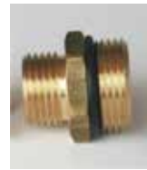
Straight fitting, brass, 3/4" side w. male thread, O-Ring and flat seat for corrugated s/s pipe, flat seat on other side.
